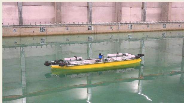
The KVLCC2 ship model performed several runs, where the ship was successfully controlled by an autopilot. The autopilots developed in the framework of the [PhD research of Changyuan Chen](#) were implemented. The system controlled the acceleration and deceleration phase based on a PID controller, performing a zigzag manoeuvre at regime speed.
