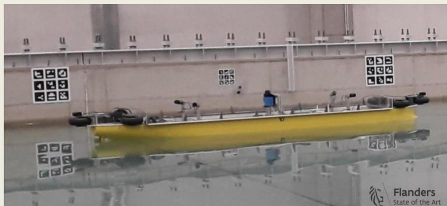
ships interacting with each other. For this type of experiments an accurate position measurement system is crucial. This is achieved by a combination of camera monitoring (towards so-called ArUco markers on the basin walls), LiDAR and gyro. The individual readings are then filtered to one position state record, which is made available for navigation routines on an on-board navigation computer. The system is expected to be production ready in spring 2022.
