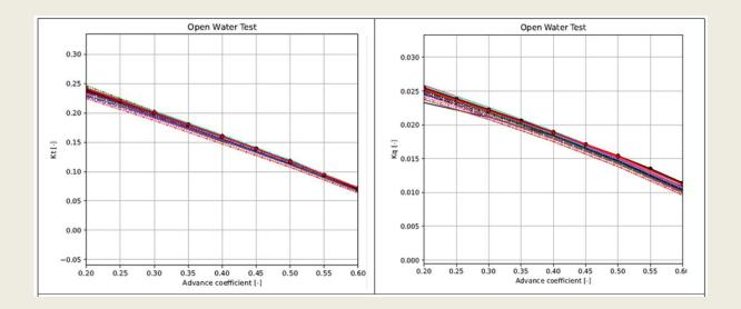
Among the workshop participants, the Maritime Technology Division of Ghent University carried out steady state numerical computations using a fine unstructured mesh containing 4 million cells. The turbulent flow was solved using the SST k-ω turbulence model which was implemented in a 3D commercial CFD solver. A moving reference frame was assigned to the fluid where the full-scale rotational speed of propeller was kept constant at 87 rpm. The computed results showed good agreement
