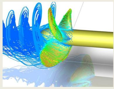
with experimental data and allowed to visualize the typical flow field around the propeller, for example to show the pressure coefficient distribution on the blade surface along with the propeller path lines coloured by velocity.
