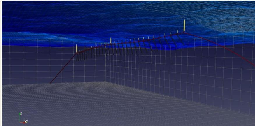
environmental loads induced by waves and current as well horizontal seabed interactions. By modelling the hydrodynamic interactions using the Morison Equation, 3-degrees-of-freedom buoys
