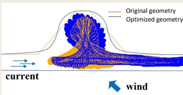
Based on a study carried out by [IMDC](#), both a circular and a trapezoidal basin were selected, with two different sizes for each. The circular geometry is built on both sides of the channel while the trapezoidal is built on one side only. Real-time simulations with a ECMT class Va and a class Va+ vessel were then carried out in different current and wind conditions. The
