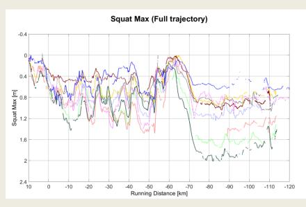
Squat motions were obtained by subtracting the steady heave and pitch motion of the vessel from the reproduced water levels and by performing a correction for draft variations due to changing water density. The squat motions of the ULCS revealed large variations which was partially related to the different operational
