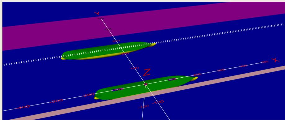
ships and wind. The potential code ROPES was first used to calculate the passing ship forces, which were then put in the software Vlugmoor, which has been developed specifically by the Division of Maritime Technology for Dynamic Mooring Analysis. Not only mooring line forces, but also motions of moored ships need to be limited, as large motions can cause delays and potential safety risks.
