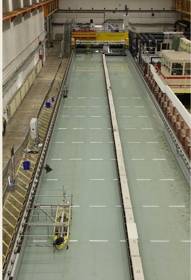
Since the planning and execution of the ROPES model tests in 2012, ship sizes have increased significantly. The capacity of the largest container ships, for example, has surpassed the 20,000 TEU mark over the last couple of years. This means that the relative size of the existing infrastructure, such as access channels, decreases. The focus of the PESCA project is to study the effect of parallel ship passages in high blockages at high passing speeds and close passing distances.
