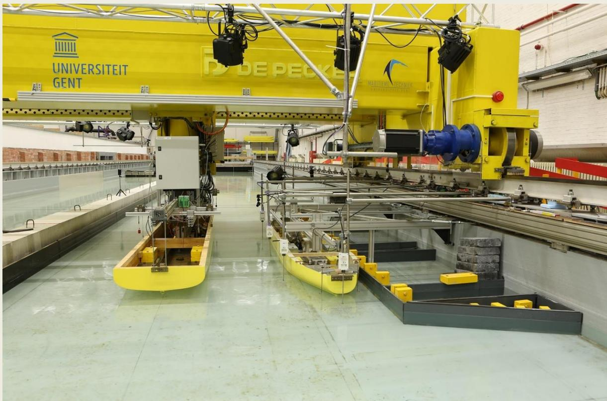
In the experiments, the blockage factor ranges from a situation in which the full tank width is used and 50% under keel clearance is present to a situation where the channel width is equal to four times the breadth of the passing ship with only 10% under keel clearance.
