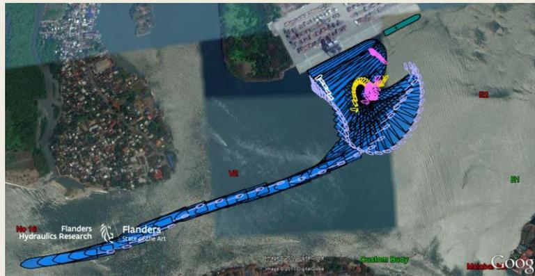
to determine the mud rheology characteristics. The results were used to adapt the mathematical model of the [manoeuvring simulators](#) at Flanders Hydraulics Research. Finally, several manoeuvres for different underkeel clearances were carried out in order to determine a safe nautical depth. The results were presented to the [Cochin Port Trust](#) to optimize their dredging strategy.
