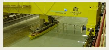
The obtained data set on <u>bank effects</u> consists of more than 14,000 unique model test setups. Different ship models have been tested in a wide range of draft to water depth ratios, forward speeds and propeller actions. The tests were carried out along several bank geometries at different lateral positions between the
