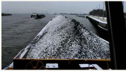
Push barge convoys have a reputation to be less manoeuvrable than conventional inland ships. The very low displacement and high wind areas of the empty barges or the large tonnage and long lengths of fully loaded combinations are some of the factors decreasing the manoeuvrability. As a result, the required path widths and turning circles can increase
